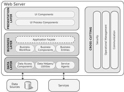
Figure 1 The typical structure of a Web application
