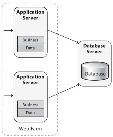
Figure 3 Load balancing a RIA deployment
