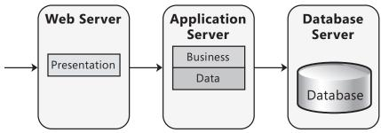
Figure 3 Distributed deployment of a Web application
