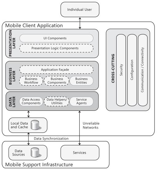
Figure 1 The typical structure of a mobile application
