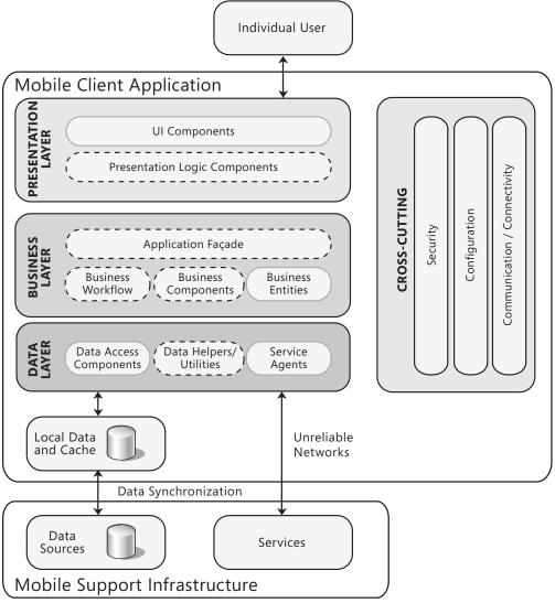
Figure 1 The typical structure of a mobile application
