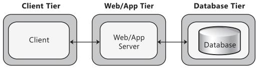
Figure 5 3-tier deployment with the application code on a separate tier
