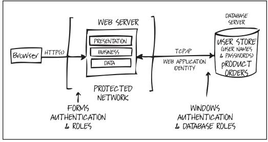
**Figure 2**Example of an architecture whiteboard showing a high-level design for a Web application indicating the protocols and authentication methods it will use.
