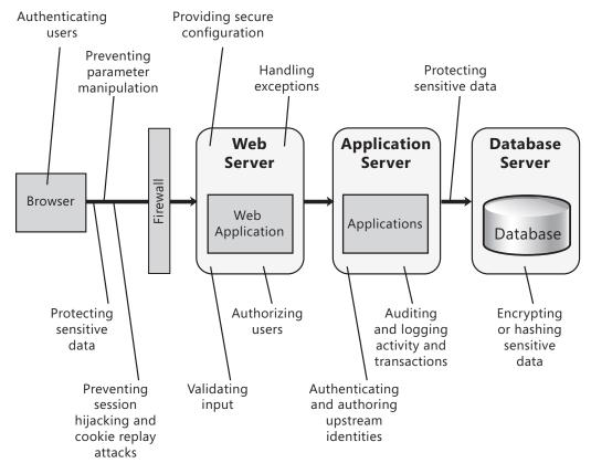
**Figure 3**Security issues identified in a typical Web application architecture.
