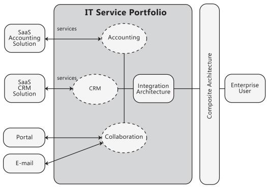
Figure 2 A service integration mechanism can compose multiple services into a single interface
