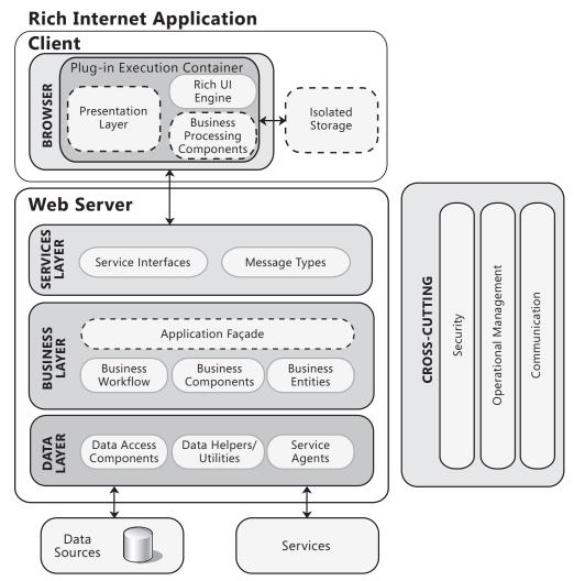
Architecture of a typical RIA implementation. Broken lines indicate optional components.
